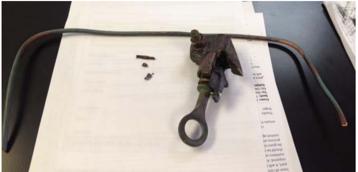
Figure 3: Worn Conductor Burnt Off Under Hot-Line Tap (Outage March 2015)
